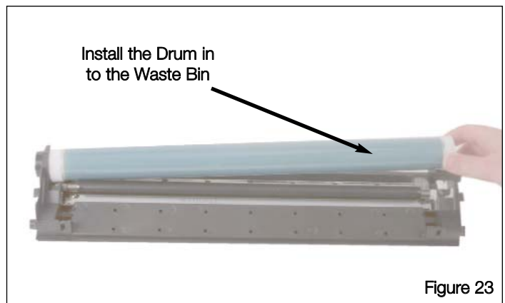
Install the drum into the Waste Bin and secure with the Drum Axle.
