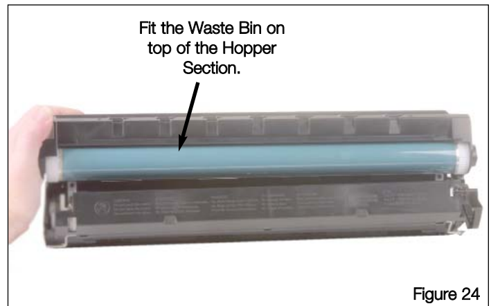
Fit the Waste Bin on top of the Hopper and secure using the 5K pins.
